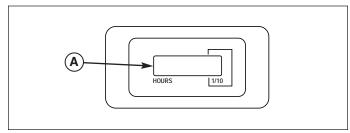
The hour meter will flash an initial oil change indicator at 5 hours, and a lubrication reminder every 50 hours. These reminders display for approximately two hours and will automatically reset themselves.
